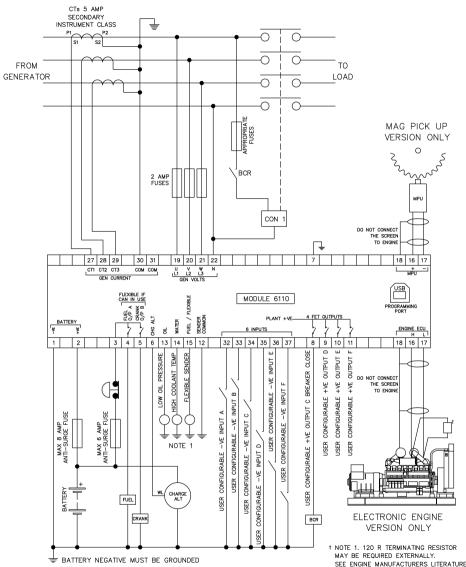
TERMINALS SUITABLE FOR 22-16 AWG (0.6mm - 1.3mm ) FIELD WIRING TIGHTENING TORQUE = 0.8Nm (7lb-in)
