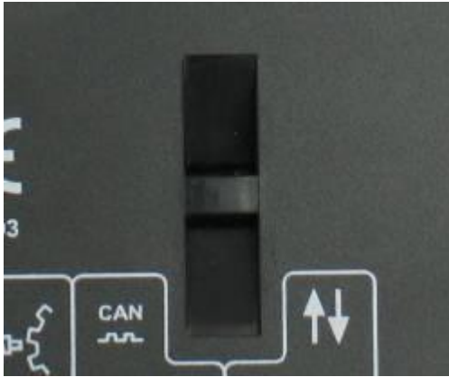
Cable Tie Fixing Point
