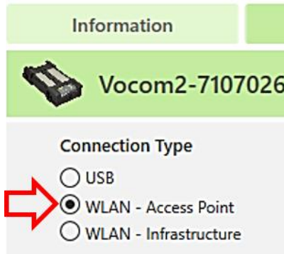
Fig. 5-8: Connection Type WLAN - Access Point
