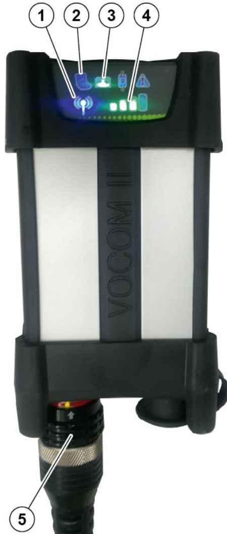
Fig. 4-2: VOCOM II function indicators in WLAN operation mode
