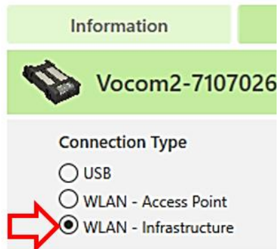
Fig. 5-15: Connection Type WLAN - Infrastructure
