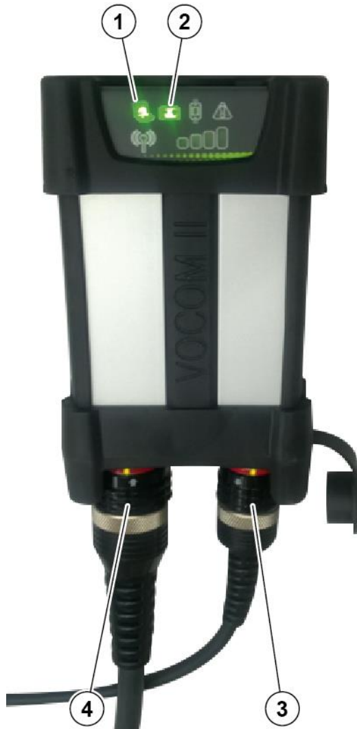
Fig. 4–5: VOCOM II function indicators in USB operation mode
