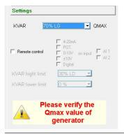
2. To set the reactive power externally, tick the box, select the source (POT, 0-10 V, etc) for this setting and also the input (Al1 or Al2). One of the inputs may be greyed-out if it is already being used by another function.
