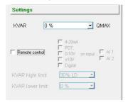
Select the value of the reactive power according to the load. This value depends on the alternator type.
