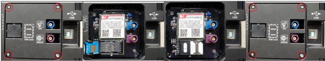
**Figure 9 – SIM Installation Steps**
