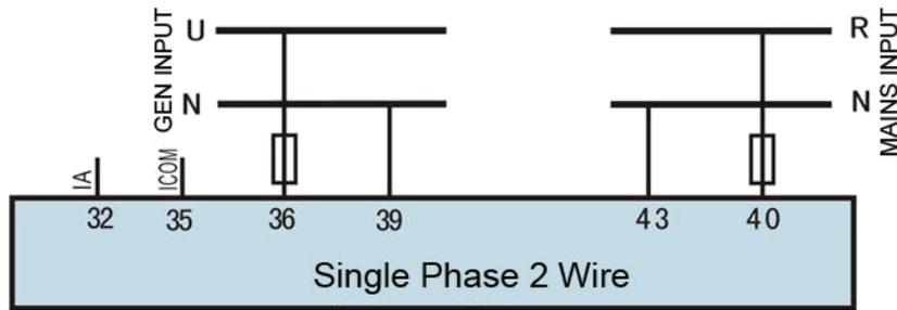
**Figure 6 - Single Phase 2-Wire Connection Diagram**
