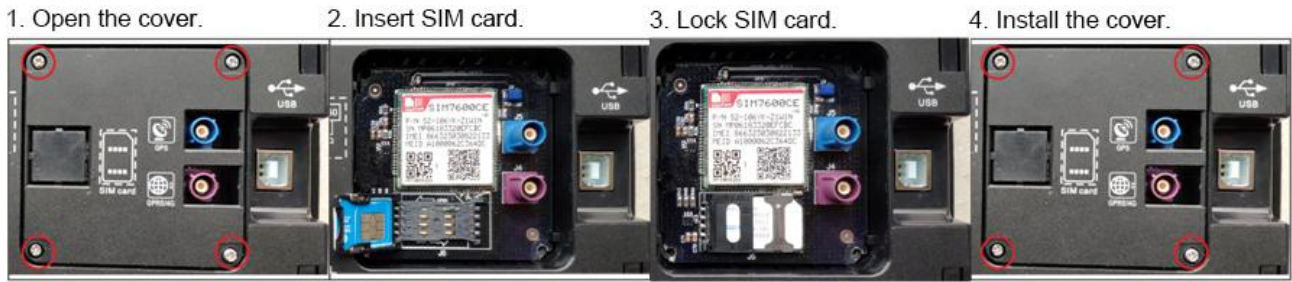
Fig. 14 SIM Card Installation Method
