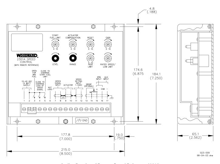
Outline Drawing of Remote Speed Reference 2301A (Do not use for construction)
