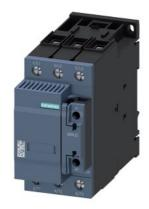
Capacitor contactor, AC-6b 50 kVAr, / 400 V 1 NO + 1 NC, 230 V AC, 50 Hz 3-pole, Size S2 screw terminal
