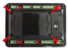
After removing back cover insert the plug-in module. Plug-in module has to be inserted under holders. Start with holders market by symbol 1. On the controller are also narrows for better navigation. After inserting plug-in module under holders 1 press it down to holders market by symbol 2 which lock the module.
