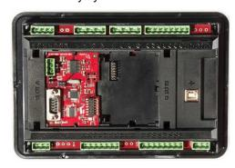
After locking the plug-in module into holders, place back the back cover (small cover for connectors has to be removed from back cover). Finally insert the small cover for connectors. Small covers are unique for each plug-in module.
