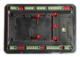
Insert the plug-in module under holders marked by symbol 1. Then insert the plug-in module under holders marked by symbol 2.
