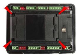
After removing back cover insert the plug-in module. Plug-in module has to be inserted under holders. Start with holders market by symbol 1. On the controller are also narrows for better navigation. After inserting plug-in module under holders 1 press it down to holders market by symbol 2 which lock the module.
