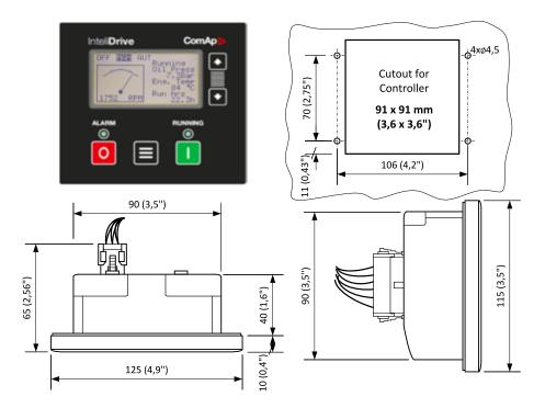
**Note:** The controller is to be mounted onto the switchboard door. The requested cut-out size is 91 × 91 mm. Use the nylon screws and nuts delivered with the controller to fix the controller into the door.
