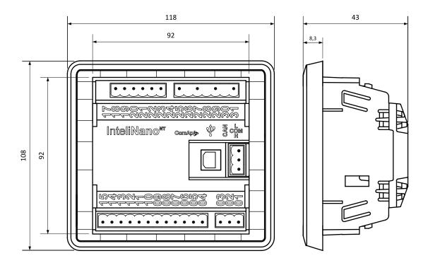
**Note:** The controller is to be mounted into panel doors as a standalone unit using provided fixing clips. The requested cut-out size is 94 × 94 mm. Use the screw holders delivered with the controller to fix the controller into the door.
