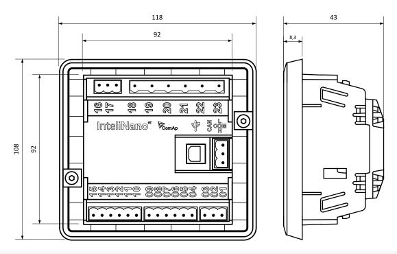
**Note:** The controller is to be mounted into panel doors as a standalone unit using provided fixing clips. The requested cut-out size is 94 × 94 mm. Use the screw holders delivered with the controller to fix the controller into the door.
