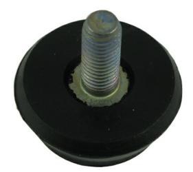
The JT-type AMC Mecanocaucho® mounts are used in cases where light or heavy machines are not fixed to the floor or ground. The height adjustment system can be used to adjust the machines to the required level, thus insulating areas nearby from vibrations and reducing noise. The AMC-Mecanocaucho® type JT comes with a tilting system accomodating uneven surfaces.
