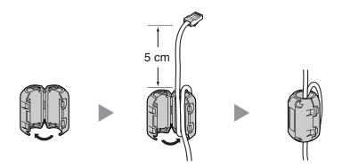
If you need to open the ferrite core, use a flathead screwdriver to unlatch the case of the ferrite core.
