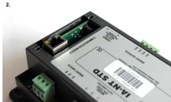
PLUGGING IN OF THE IB-LITE COMMUNICATION MODULE
