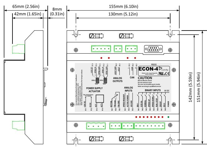
**Note:** The unit is mounted on DIN rail (35 mm/1.38 in).
