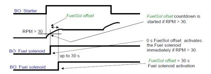
**Note:** A new feature has been added which prolongs the last cranking attempt by 25% of MaxCrank time with closed Fuel valve (Fuel Solenoid binary output) in order to ventilate the remaining gas, as is implemented in IG/IS-NT. This function is valid only when **Fuel solenoid (page 117)** = GAS
