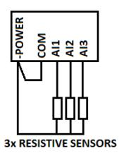
Standard connection of three resistive sensors to analog inputs.
