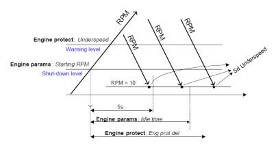
Tables below describe Underspeed protection behavior depends on Underspeed Sd setpoint setting and RPM value.
