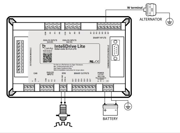
**Note:** The RPM-BI3 measuring is switched off when Basic setting: GearTeethBI3 = 0. In this case BI3 operates as standard Binary input.
