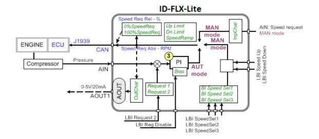
Following example changes the RPM between two levels based on pressure.
