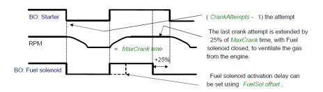
**Note:** Is modified functionality of the Ignition binary output. The Ignition binary output will close 1 second (fixed value) after activation of binary output Fuel solenoid (when Fuel solenoid = GAS setting is active). Generally, the output closes after reaching value of CrankRPM = 30RPM (fixed value). The output opens after stopping of the engine or during crank fail pauses among crank attempts.
