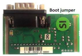
Boot jumper programming – In case of interrupted programming or other software failure is possible to use the boot jumper programing to restore controller to working order. Connect the controller to PC, run LiteEdit and wait until connection bar at bottom turns red. Than run programming process via menu Controller -> Programming and cloning – Programming. Select correct firmware and confirm dialog. Than follow instructions in LiteEdit.
