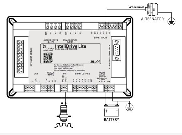
**Note:** The RPM-BI3 measuring and corresponding protections are switched off when **GearTeethBI3** (page 98) = 0. In this case BI3 operates as standard binary input.
