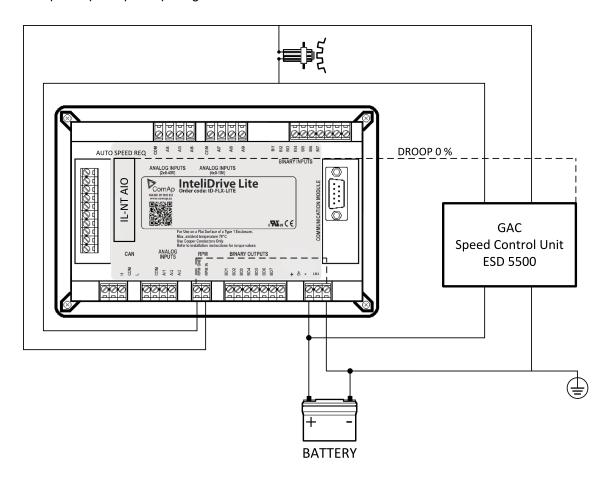
Note: If RPM > 2 then the controller is in the state Not ready and the engine will not be allowed to start.
