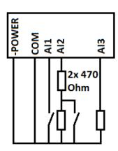
Mixed connection of ID-Lite analog inputs:
