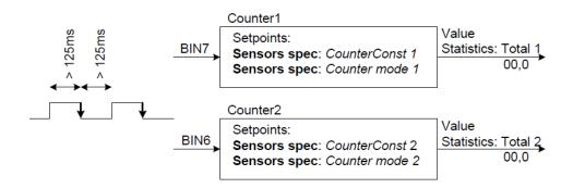
Counter 1 (fix linked to Binary physical input 7) and Counter 2 (fix linked to Binary physical input 6) counts pulses (falling edges). The counters function depends on Counter mode 1 and  $\dots$  2 setting and does not depend on BIN6, BIN7 inputs configuration. The maximal input frequency is limited op to 4 Hz – i.e. the shortest input pulse is 125 ms and gap 125 ms (not shorter) to be each edge counted.
