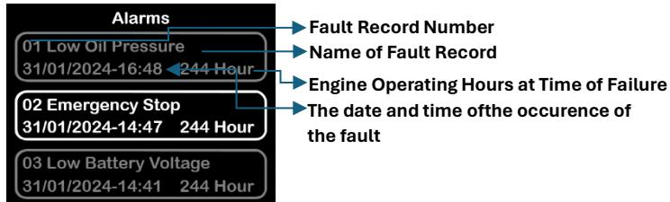
Navigate to the "EVENTS AND ALARMS" heading from the main menu and press the enter button. You can access the last 50 event records by selecting "Events" and pressing the enter button, or the last 50 alarm records by selecting "Alarms" and pressing the enter button. The records include time information in day, month, year, hour, and minute format; the generator's operating hours at the time of the event are also recorded.
