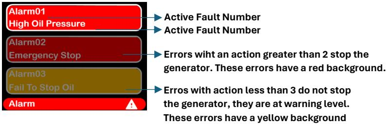
From the main screen, use the right and left navigation buttons to go to the active alarms page. Alarms are listed with a red or yellow background. Alarms with a yellow background are at a warning level and do not stop the generator, while alarms with a red background can stop the generator. You can delete an alarm you wish to clear by navigating to it and pressing the alarm silence button.
