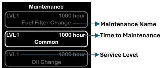
From the main menu, go to the "MAINTENANCE" option and enter by pressing the enter button. After selecting the service interval to be reset using the up and down navigation buttons, hold the enter button for 5 seconds to reset it.
