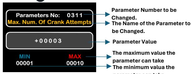
Press the enter button to activate the parameter number selection. Use the navigation buttons to input and confirm the desired value with the enter button. Then, press the down navigation button to move to the set value field, enter the password screen with the enter button, and proceed if the password is correct. Confirm the new parameter value using the navigation buttons and finalize it with the enter button. To exit the parameter menu, hold the left navigation button for 1 second.
